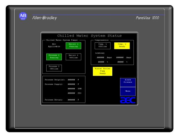
The Chiller Status screen shows the status for compressors within the system. Only compressors that are included in the system will be shown on this screen. Compressors will display one of the following states:
